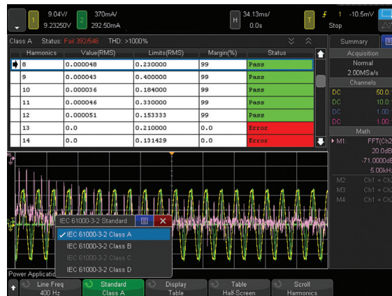
Figure 2. Perform the pre-compliance line harmonic testing of your power supply to the IEC 61000 3-2 standards. This analysis presents up to 40 harmonics.
