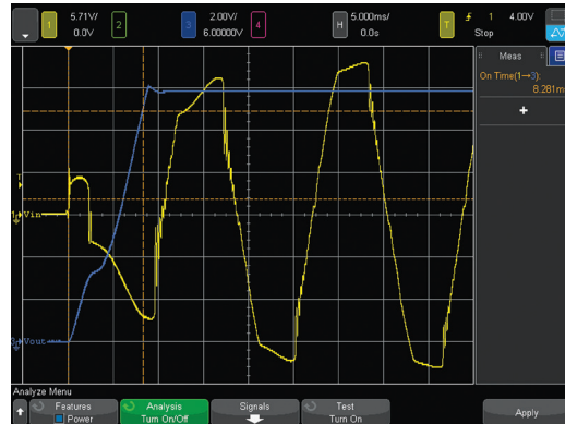
Figure 7. The turn-on analysis measures the time taken to get to the steady output voltage of the power supply after the input voltage is applied.
