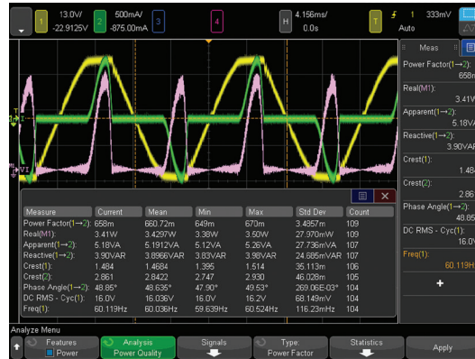
Figure 4. The power measurements option provides a results table with the following power quality measurements: Power Factor, Real Power, Apparent Power, Reactive Power, Crest Factor and Phase Angle.
