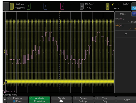
Figure 5. Plotting the embedded variation of on time or off time in the PWM signal over a long period of time can reveal the control loop response of the feedback loop system.
